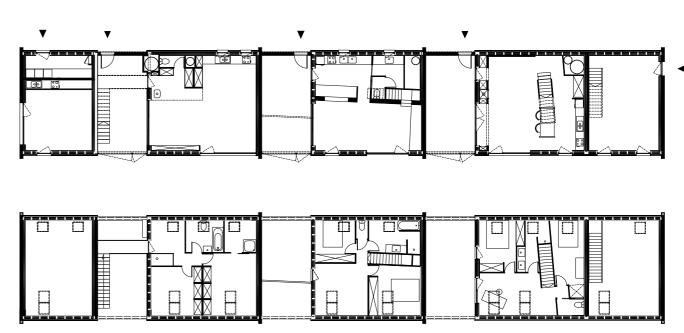
Above: floorplan of the ground floor, from the left: common area with laundry, apartments, office. The northern walls of the greenhouses are partially massive to prevent heat loss, while the rest, including roof, is cladded in polycarbonate. The garden facades are divided in two elements, which – thanks to hinges on both sides – can be folded for ventilation. The middle apartment features a heating wall made out of rammed earth.
